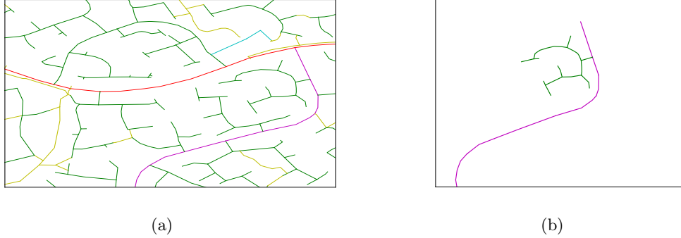
Figure 1: A section of street network from OSM London. (a) Five different road classes can be seen: secondary (red), tertiary (magenta), residential (green), footway (yellow), service (cyan). (b) Two connected sets of street segments, one each from tertiary and residential classes have been redrawn for comparisons.
