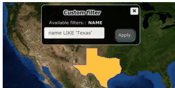
Figure 9: CQL filtering example. In this example, the layer that displays the state boundaries for the U.S. is filtered to show only the state of Texas.
