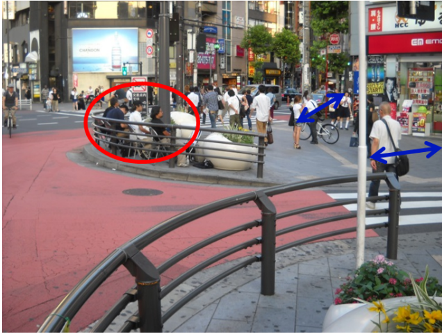
Figure 8: Snapshot of pedestrian traffic census in Roppongi Intersection area. Survey crews are indicated with red circles. They counted pedestrians passing the blue segment, which are D and E segments in Figure 7.
