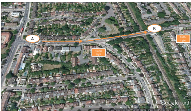
Figure 9: Locations of the upstream sensor A and the downstream sensor B. Cars move from A to B. Between A and B there is a junction. Most of the flow from A moves further to B.
